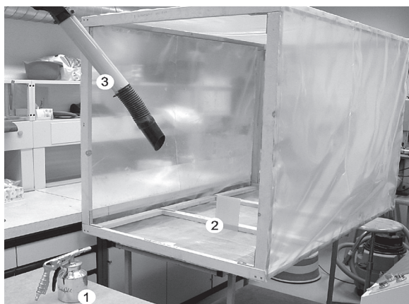
Fig. 1.3. Substance application chamber: In front the dust spray gun (1) and in the chamber the Plexiglas support (2). The tube is the dust extraction unit (3) (for working safety reasons)
